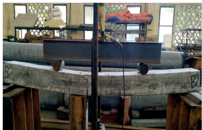
Figure 8. Views of the destruction of the tested beam samples
