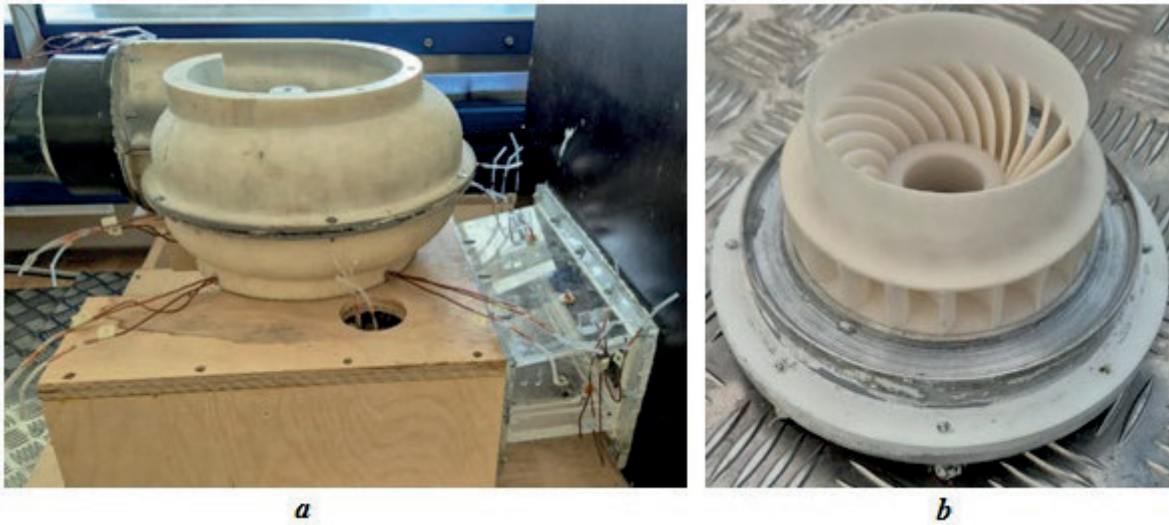
Figure 3. Turbine block model: a – general view, b – turbine cover with counter-vortex damper
