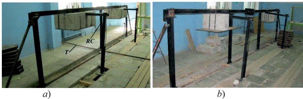
Figure 3. General view of experimental specimens: (a) with rigid assemblies; (b) with hinged assemblies (showing the erecting supports used before installing the middle column)
