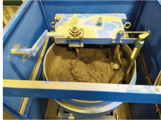
Figure 1. Production of concrete mix
