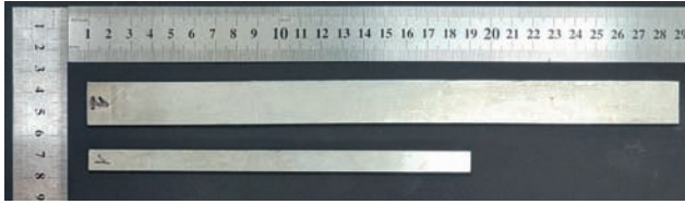
Figure 1. The types of TPCM samples under study are from the top a sample measuring 280mm x 20mm x 0.8mm and from the bottom a sample measuring 180mm x 10mm x 0.8mm
