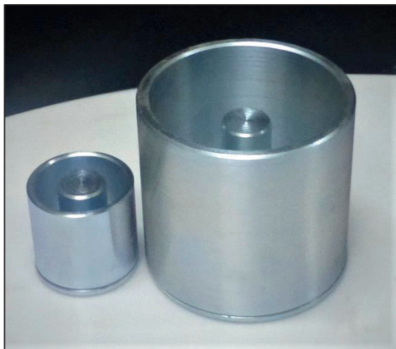
a) Russian Cylinders \varnothing 75 and \varnothing 150 mm
