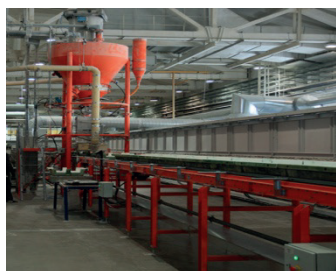
Figure 2. Loading the raw material mixture into the molds
