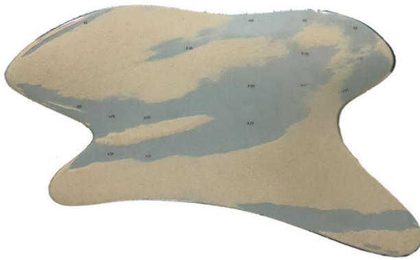
a) distribution of the snow simulator after blowing
