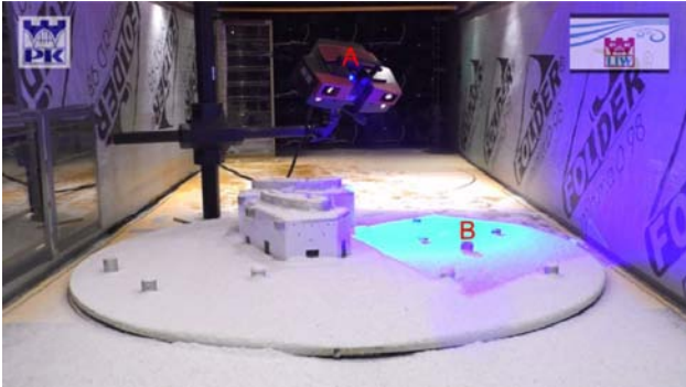
b) the process of 3D scanning of the experimental results
