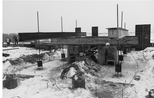
Fig. 1. Typical static load test (SLT)
