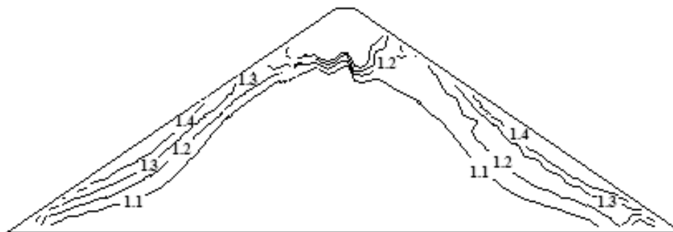
Figure 2. Distribution of isolines of safety factor K in the body of homogeneous dam.
