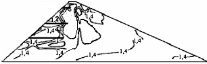
Figure 4. Distribution of isolines of safety factor) K in a dam at \varphi=30^\circ , C=0 with laying of upper slope m_1=1 , m_2=2 at irregular ( 0.4H , 0.6H and 0.9H ) location of anti-seismic reinforced concrete seismic belts.
