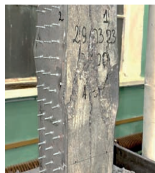
b) characteristic failure
