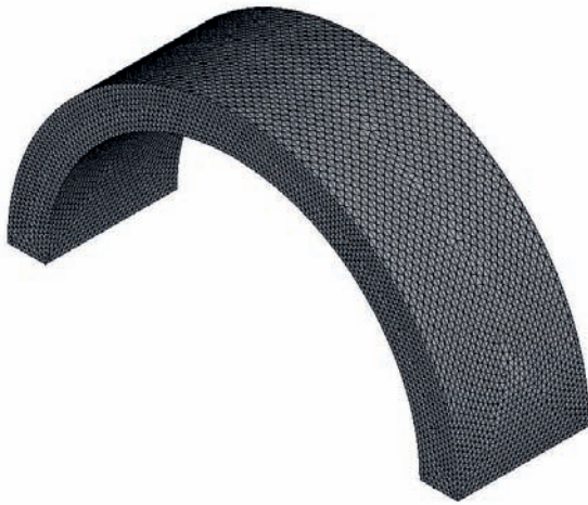
Figure 2. Discretization of the shell on the FE
