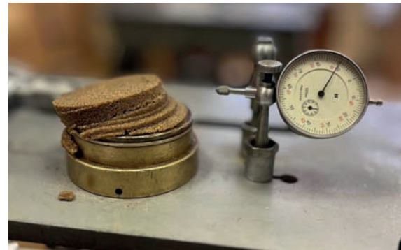
Figure 3. Sandy soil sample contaminated with diesel fuel after the single plane shear test
