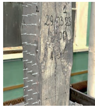
b) characteristic failure
