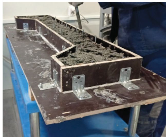
Figure 2. Compacting fresh concrete with tamper and vibration on laboratory vibrating table
