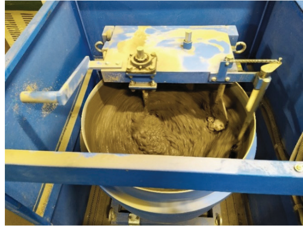
Figure 1. Production of concrete mix
