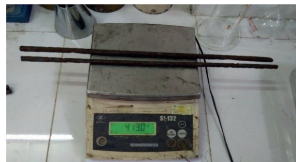
Figure 8. Weigh the reinforcement sample to determine the level of corrosion
