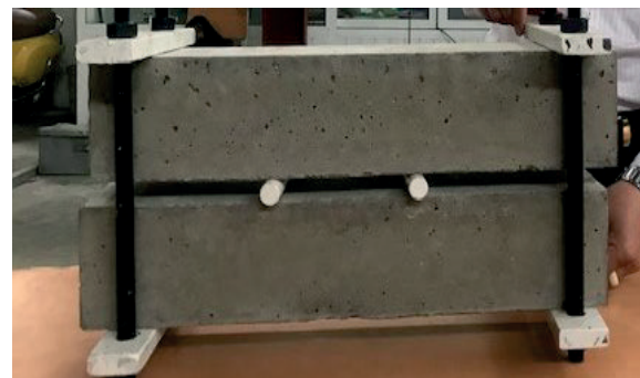
Figure 4. Loading beams for beam samples
