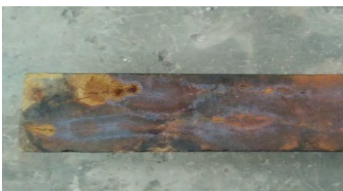
Figure 6. Sample after immersion in accelerated corrosive environment
