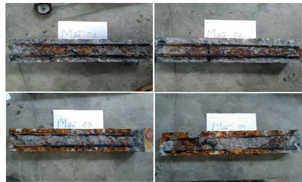
Figure 7. Steel reinforcement is corroded after removing the concrete layer
