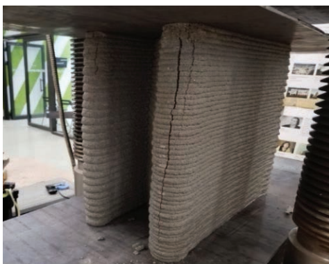
Figure 6. A representative example of the 3D-printed-size wall segments during the compressive strength test
