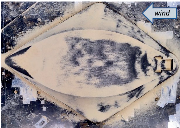
a) physical modelling for wind direction 90° (surrounding buildings ignored)
