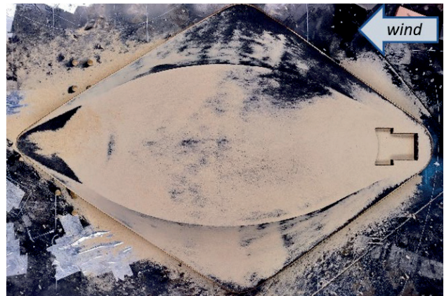
b) physical modelling for wind direction 90° (surrounding buildings considered)
