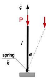
Figure 18. Transition of a rod to the deflected state during buckling.
