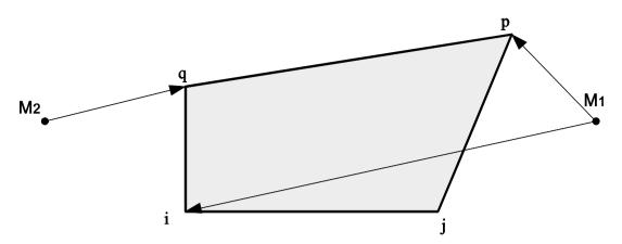
*Figure 2.* Four-node shell finite element with imposed rigid links.  $M_1$ ,  $M_2$  are master nodes.
