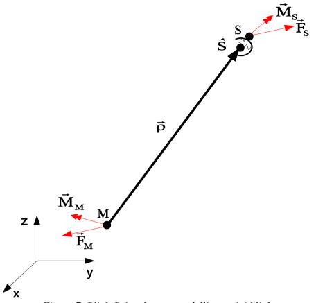
Figure 7. Rlink finite element modelling a rigid link.
