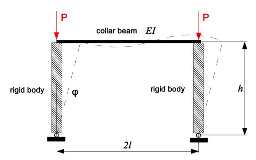
*Figure 3.* Design model of a plane frame with rigid columns. Dashed line shows the buckling mode.
