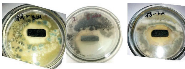
Figure 9. Degree of mold growth on concrete with a Glenium plasticizer with PHMG additive dosage: 7 – 0%; 4 – 0,5%C; 9 – 2%C
