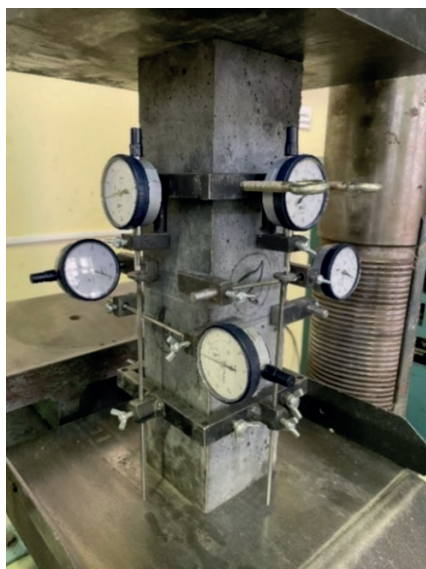
Figure 1. Tests of prism specimens with determination of the static elasticity modulus and Poisson's ratio of concrete on a hydraulic press
