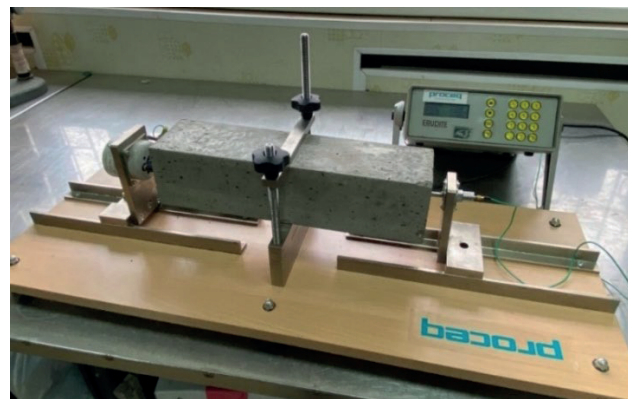
Figure 2. Tests of prism specimens with determination of the dynamic elasticity modulus of concrete using the Erudite MKIV (PC 1004) device
