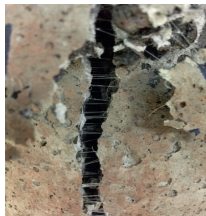
Figure 6. Location of fibers within the crack at the moment of complete failure (see Fig. 3, c)
