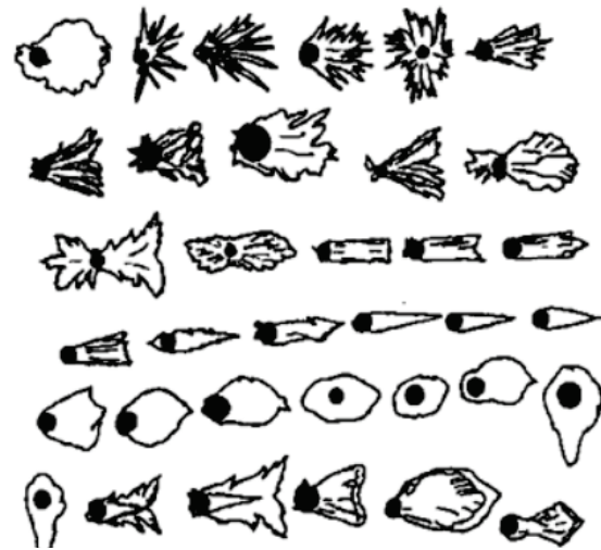
Figure 5. Possible forms of ice deposits on wires
