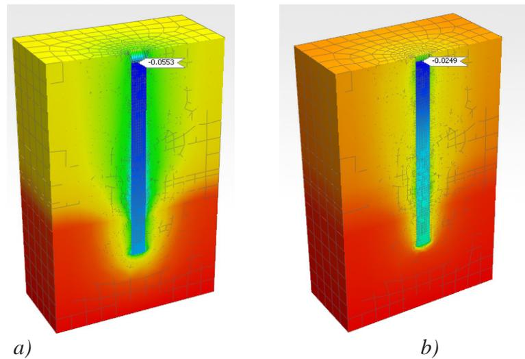
Figure 3. Deformed diagram and vertical displacements of the model under a load of 20,000 kN: a) Mohr-Coulomb model, b) Hardening Soil model
