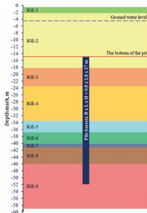
Figure 1. Layout of the pile-barretts in the ground
