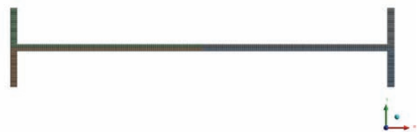
Figure 4. Computational grid for CSD model: Model 4 (10 913 nodes).
