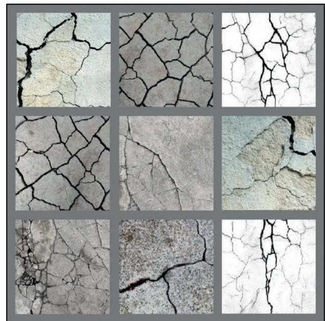
Figure 1. Some examples of the crack-damaged concrete surfaces
