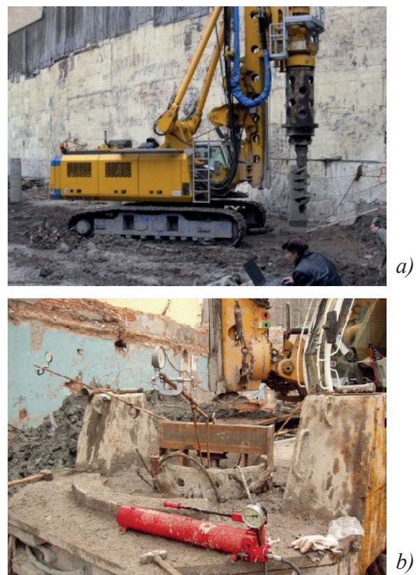
Figure 5. The complex science investigations on the construction site: taking vibration measurements during the construction of drilled cast-in-situ piles (a); the stamp test of the soil on the bottom pile's level (b).
