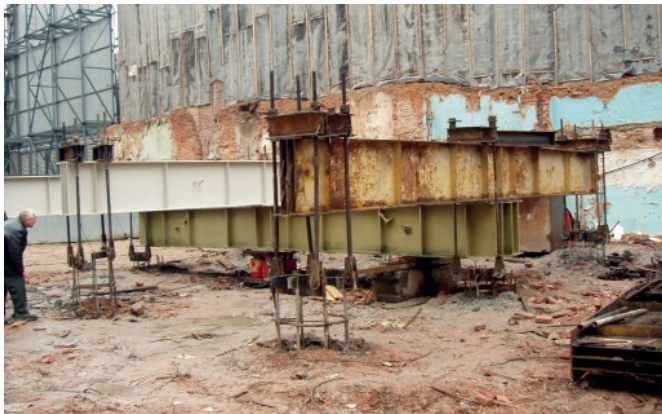
Figure 6. Static tests of piles using hydraulic jacks
