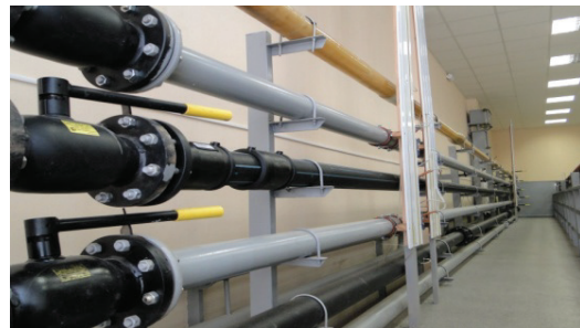
Figure 1. General view of a large-scale hydraulic test rig with 10 m long pipes with a nominal diameter of 100 mm made of various materials (the fourth pipe from the top is a steel pipe with a protective Subcote FLP coating)
