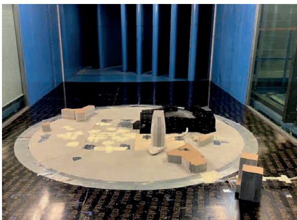
Figure 3. MTEC model in the MSUCE WT (control points are coloured white)
