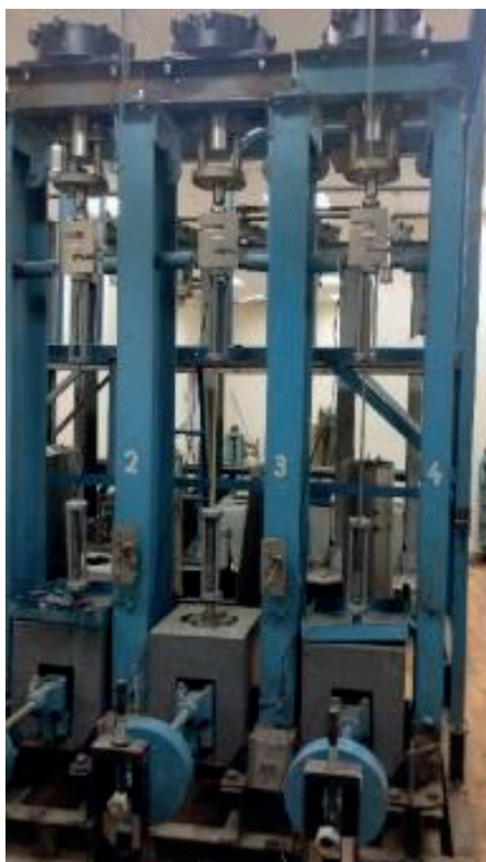
Figure 1. General view of long-term testing of FRP bar specimens (before test stand modernization)
