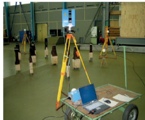
Figure 9. Laser-scanning setup for post-fire residual cross-section measurement
