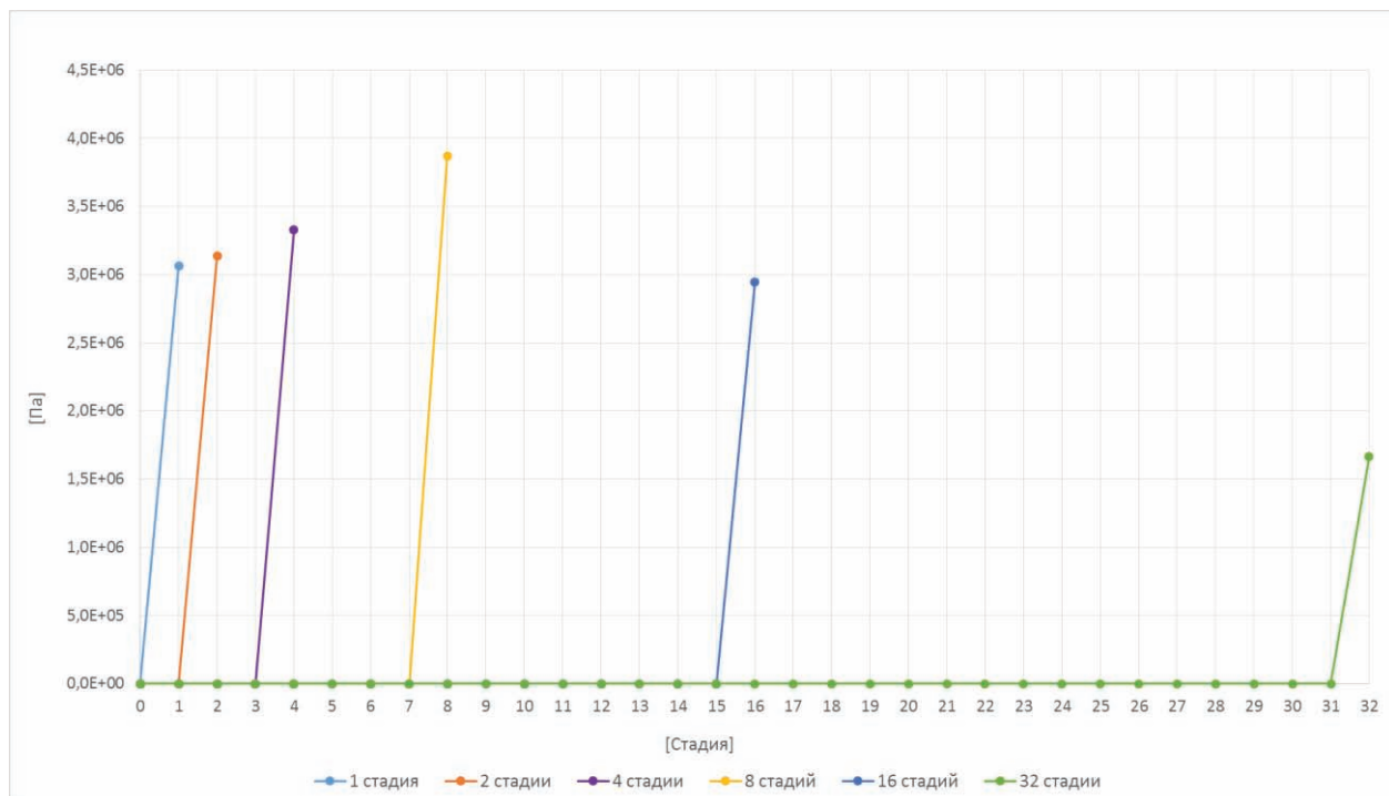
Figure 10. The maximum equivalent stresses according to the IV strength theory (von Mises) of 32 ring of the shell.
