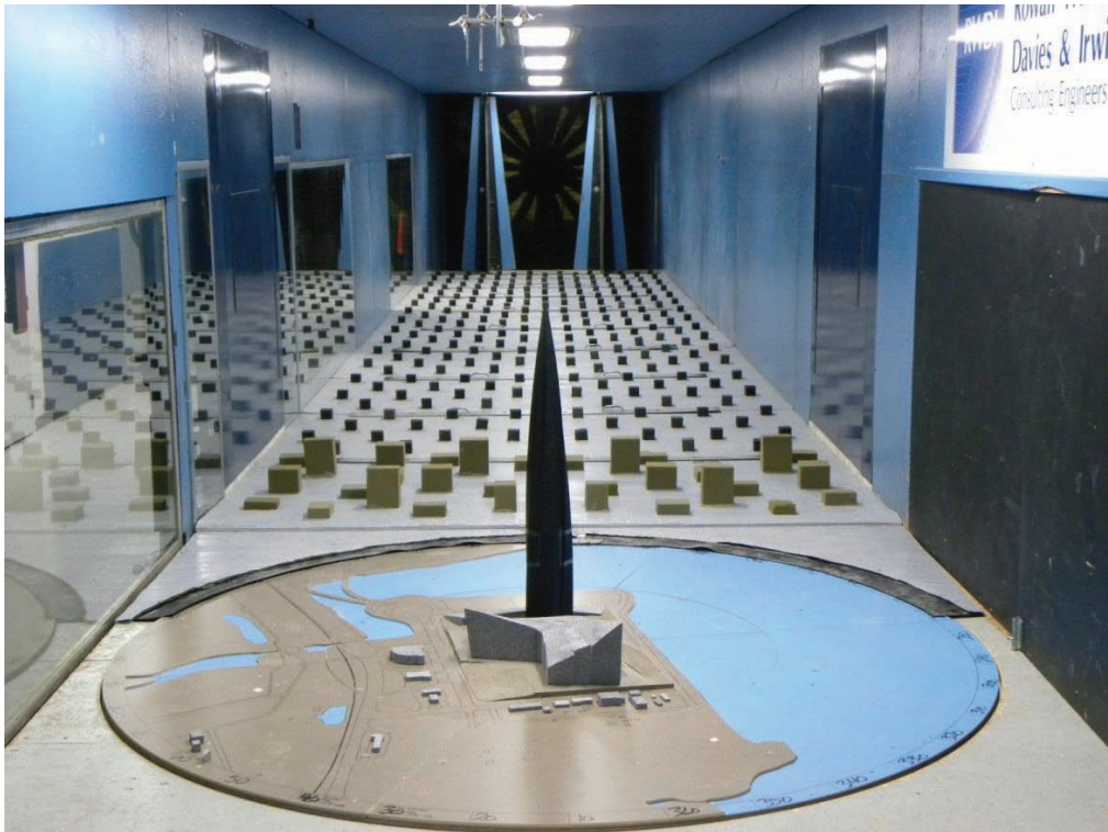
Figure 21. View of the Lakhta Center model in the RWDI wind tunnel.
