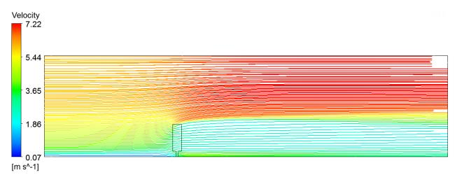
Figure 3. Velocity stream lines, m/s. Volume porosity  $\gamma = 1$ , loss coefficient  $K_{loss} = 1.75$ .
