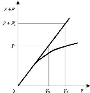
Figure 1. Scheme of the method of elastic decisions which is used by AFEM for the allowance of the first nonlinear property when its additional load is  $F_{e,l} = -\Delta R_{nonl,l}$  [20,21].
