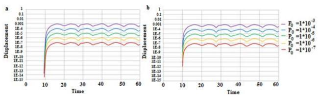
*Figure 3.* Displacement on the free surface for p.1 when a)  $\Delta x = 0.05$ , b)  $\Delta x = 0.01$ .
