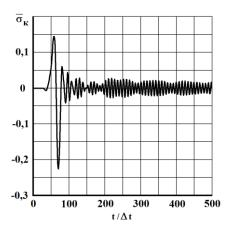
Figure 9. Change of elastic contour stress  $\bar{\sigma}_k$  in time  $t/\Delta t$  at the point A5.
