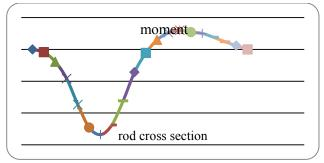
Figure 3.8. Diagrams of deflections and bending moments for  $\alpha = 3,976$ ,  $v_1 = 0,2$  and  $v_2 = 0,6$  ( $\Delta = 0,2$ ).
