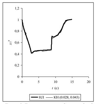
Figure 9. Transition process for normalized control variable  $x_5^n$  nonlinear (NL) model and discrete-continuous (DC) model, corresponding to wide range of operation modes of nonlinear control object.
