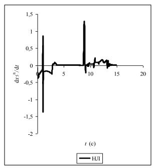
Figure 10. Transition process for derivative of the normalized control variable  $x_5^n$  of nonlinear (NL) model, corresponding to wide range of operation modes of nonlinear control object.
