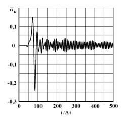
Figure 13. Change of elastic contour stress  $\bar{\sigma}_k$  in time  $t/\Delta t$  at the point A9.
