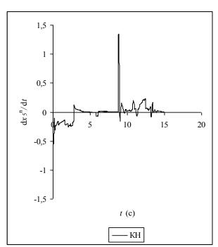
Figure 12. Transition process for derivative of the normalized control variable  $x_5^n$  discrete-continuous (DC) model, corresponding to wide range of operation modes of nonlinear control object.
