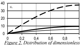
displacement  $u_*$  along the length of a beam.
