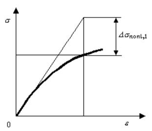
Figure 2. Scheme of the method of additional stresses which is used by AFEM for the allowance of the first nonlinear property by means of AFE of the first type [19, 20]
