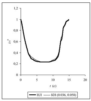
Figure 8. Transition process for normalized control variable  $x_4^n$  nonlinear (NL) model and discrete-continuous (DC) model, corresponding to wide range of operation modes of nonlinear control object.
