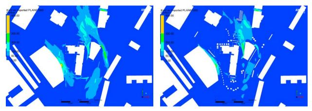
Figure 10. 2nd level of pedestrian comfort  $V_{cr2}=12$  m/s exceeding no more  $K_{cr2}=50$  hours per year in the pedestrian zone at a height of 1.5 m (on the left - without bushes, on the right - with bushes).
