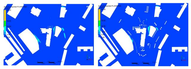
Figure 11. 3st level of pedestrian comfort  $V_{cr3}$ =20 m/s exceeding no more  $K_{cr3}$ =5 hours per year in the pedestrian zone at a height of 1.5 m (on the left - without bushes, on the right - with bushes).
