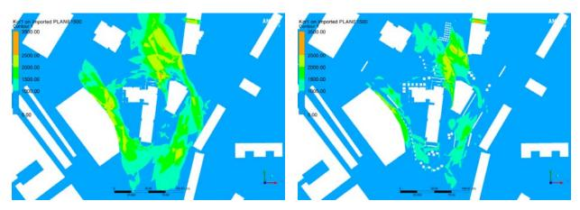
Figure 9. 1st level of pedestrian comfort  $V_{cr1}$ =6 m/s exceeding no more  $K_{cr1}$ =1000 hours per year in the pedestrian zone at a height of 1.5 m (on the left - without bushes, on the right - with bushes).
