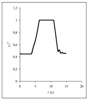
Figure 2. Transition process for normalized control variable  $u_2^n$ , corresponding to wide range of operation modes of nonlinear control object.
