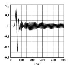
Figure 7. Change of elastic contour stress  $\overline{\sigma}_k$  in time  $t/\Delta t$  at the point A3.
