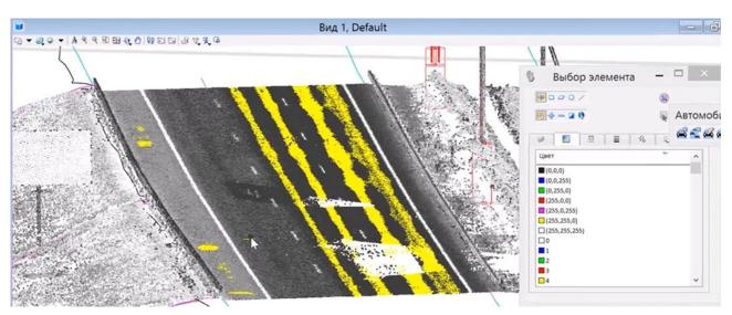
Figure 4. The result of laser scanning with subsequent analysis of the road pavement.
