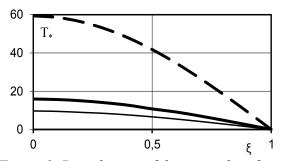
Figure 3. Distribution of dimensionless force  $T_*$  along the length of a beam.
