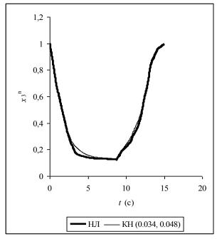
Figure 7. Transition process for normalized control variable  $x_3^n$  nonlinear (NL) model and discrete-continuous (DC) model, corresponding to wide range of operation modes of nonlinear control object.
