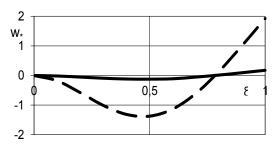
Figure 4. The deflection  $\mathbf{w}_*$  as a function of the coordinate  $\xi$  near the second resonance of the beam at  $\lambda_2 = 4.693$ .
