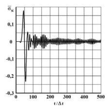
Figure 5. Change of elastic contour stress  $\overline{\sigma}_k$  in time  $t/\Delta t$  at the point A1.
