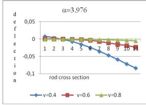
Figure 2.2. Diagrams for comparison deflections of the beam at length decreasing of supported part of the beam.
