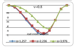
Figure 2.5. Diagrams of bending moments for different combinations of damage sizes (1-v).
