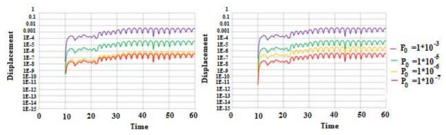
*Figure 5.* Displacement on the free surface for p.1 when a)  $\Delta x = 0.05$ , b)  $\Delta x = 0.01$ .
