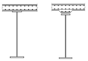
a) slab withoutb) slab with thickening
