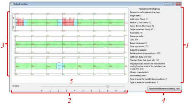
*Figure 3.* Window for displaying the state of the road with the display of problem areas.
