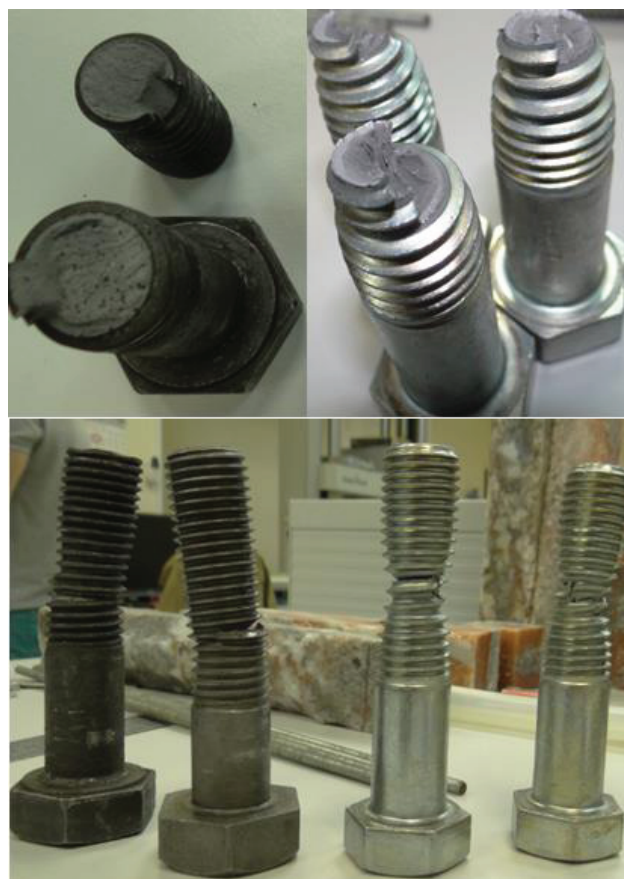
Figure 6. Characteristic destruction of bolts. On the left – bolts 10.9 from steel 40Kh, on the right – bolts 8.8 from steel 20G2R.
