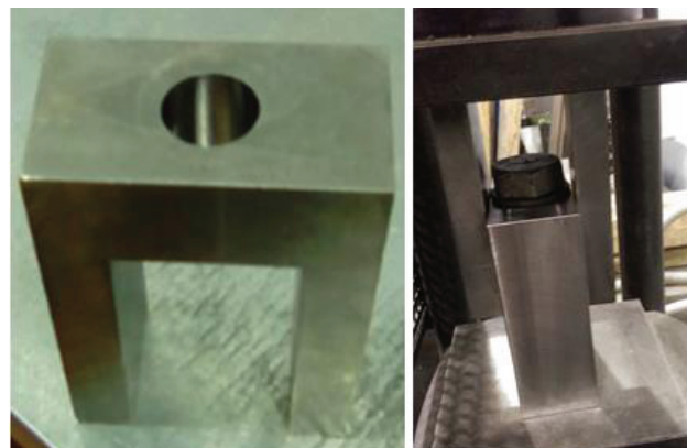
Figure 3. On the left – part of reverser, on the right – bolt test in press, using reverser.
